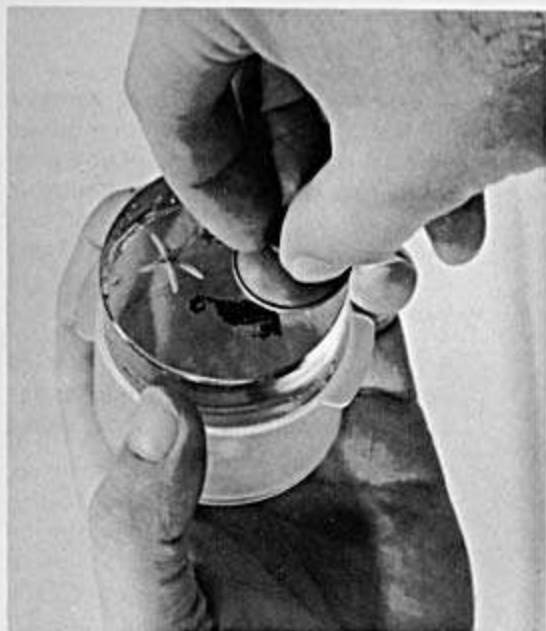
Here the cured mould piece is removed with a rubber suction pad. Careful tapping or strong cooling is always better than any type of force.
