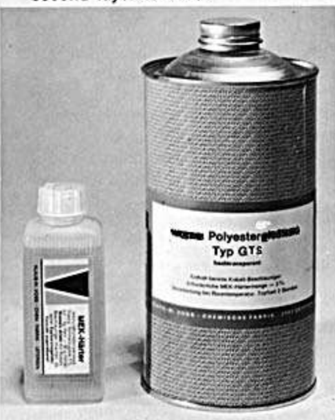
Casting resin GTS is a faint green in its liquid state. During curing it suddenly becomes transparent, shortly before gelation.
