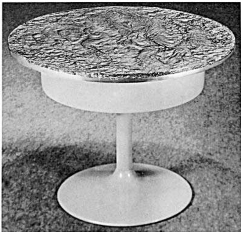
This round aluminium plate was cast by a special process and had a matt finish. A frame was placed around the plate about 1 cm (under ½ in) deep and resin poured into it. It was then polished.
