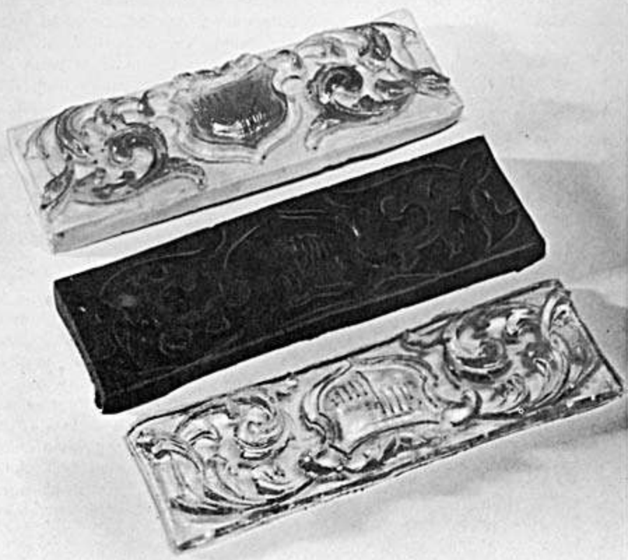
The middle mould was made from the original with Silicone Rubber. The top piece was potted in two layers, the first layer being coloured green.
